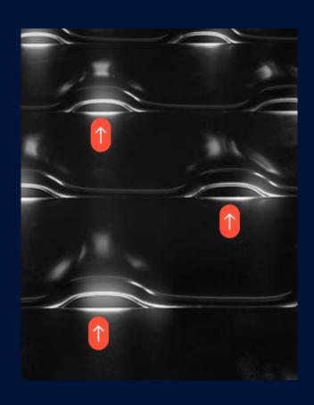
**CONIDUR®** hole sheets are applied as screening/separation screens in mills. The milling process is aided by the roughness of the working side. The special conical hole shape reduces blinding through near mesh particle.
